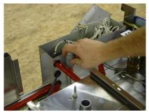
7. Electrical box front is free to move, angle it forward while shifting it to the side.
