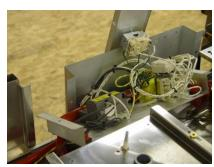
8. Loosen the screws holding the spark module in place and remove the module.
