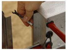
6. Remove both 7mm screws at box front base.
