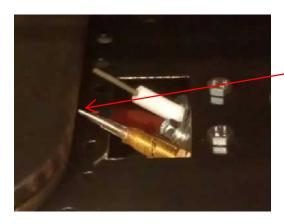
The tip of the thermocouple should NOT touch the burner
